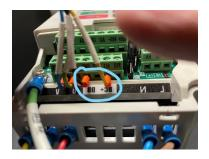
3) Connect one of the outside posts of your switch with a segment of yellow wire back to the Al1 post on the VFD. This is to operate the VFD and spindle.
